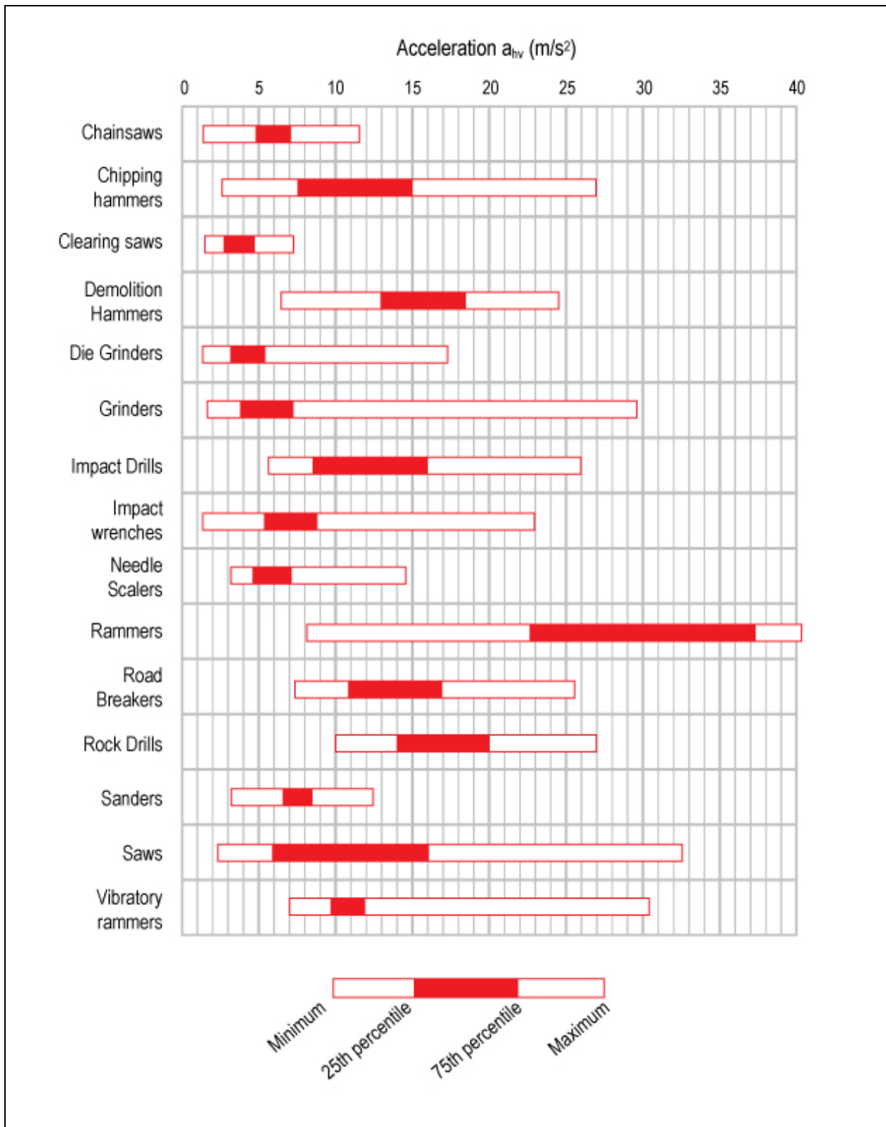
Figure 3 - Typical Hand-Arm Vibration Intensities for Various Hand-Tools (Data from the Hand-Arm Vibration Guide , Griffin et al, 2006)
